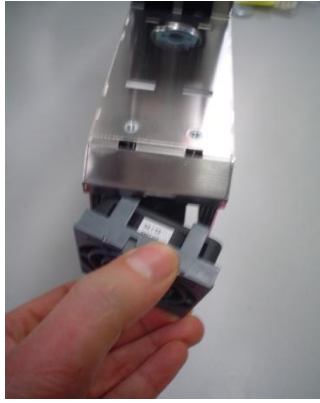
Figure94Replacingthe drives' cooling fans 更换驱动器的散热风扇
