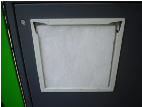
Figure 66:Checking and replacing the dust filter 检查和更换滤尘器
