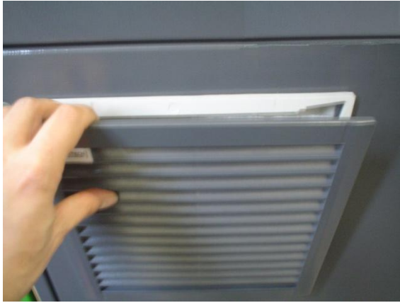
Figure 65:Checking and replacing the dust filter 检查和更换滤尘器
