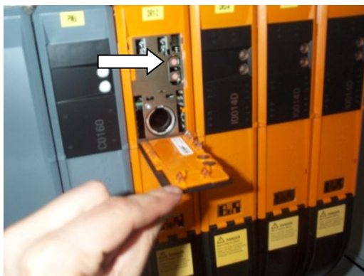
Figure 90: Replacing a drive 更换驱动器
