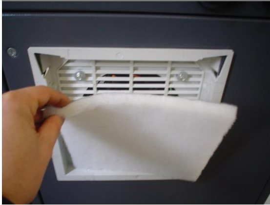
Figure 67: Checking and replacing the dust filter 检查和更换滤尘器
