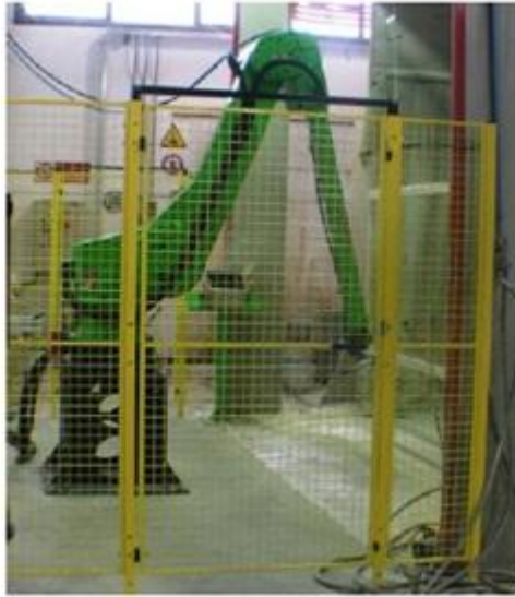
Figure 76: Perimeter fence 防护围栏
